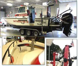
**Fittings/hardware:** Powder coated (black) bow rails, exterior and interior cabin grab rails, cleats, stern rails, navigation light mast - fuel & foam tank fill fittings - transom chafe cap - self draining scuppers. Also see next page for fire fighting equipment
