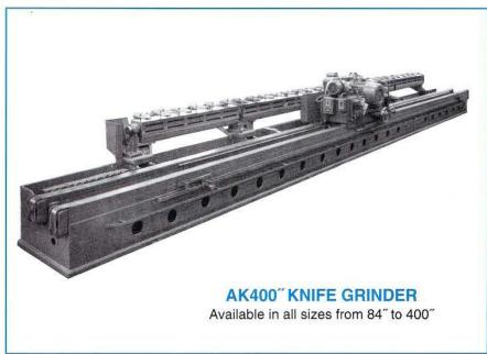
An infinite number of bevel angles can be easily set up with the adjustable knife bar. The rugged 8" square knife bar is completely adjustable for 360° through a worm gear pivot mechanism. Standard knife bars have "T-bolt" slots for clamps and are finished on four sides, providing large work areas capable of accepting different part sizes. Special bars offering hydraulic, pneumatic or magnetic clamping devices are available as optional equipment.
